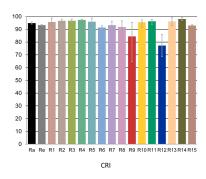
Work equipment Adjustable electronic ballast, digital DALI **Connected load** 220 - 240 V; AC; 50 Hz; 60 Hz **Power consumption** ca. 46 W Standby ca. 0,25 W Luminous flux approx. 6.200 lm Luminous efficiency 1) approx. 134 lm/W Light type/-color adjustable white approx. 2.700 - 6.500 K Colour temperatur Color rendering index  $CRI \ge 90; R9 \ge 50$ Light distribution Direct/indirect **Chromaticity tolerance LED** < 3 SDCM UGR class (4H 8H; EN 12464-1) ≤ 22
