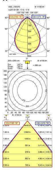
Work equipment Electronic ballast **Connected load** 220 - 240 V; 50 Hz; 60 Hz **Power consumption** ca. 30 W Standby ca. 0,5 W Power factor env. 0,900 Luminous flux approx. 4.100 lm Luminous efficiency 1) approx. 136 lm/W Light type/-color Cold white
