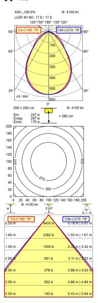
Work equipment Electronic ballast **Connected load** 220 - 240 V; 50 Hz; 60 Hz **Power consumption** ca. 30 W Standby ca. 0,5 W Power factor env. 0,900 Luminous flux approx. 4.100 lm Luminous efficiency 1) approx. 136 lm/W Light type/-color Cold white Colour temperatur approx. 4.000 K
