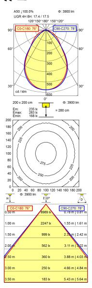
Work equipment Electronic ballast **Connected load** 220 - 240 V; 50 Hz; 60 Hz Power consumption ca. 30 W Standby ca. 0,5 W Power factor env. 0,900 Luminous flux approx. 3.900 lm Luminous efficiency 1) approx. 130 lm/W Light type/-color Warm white
