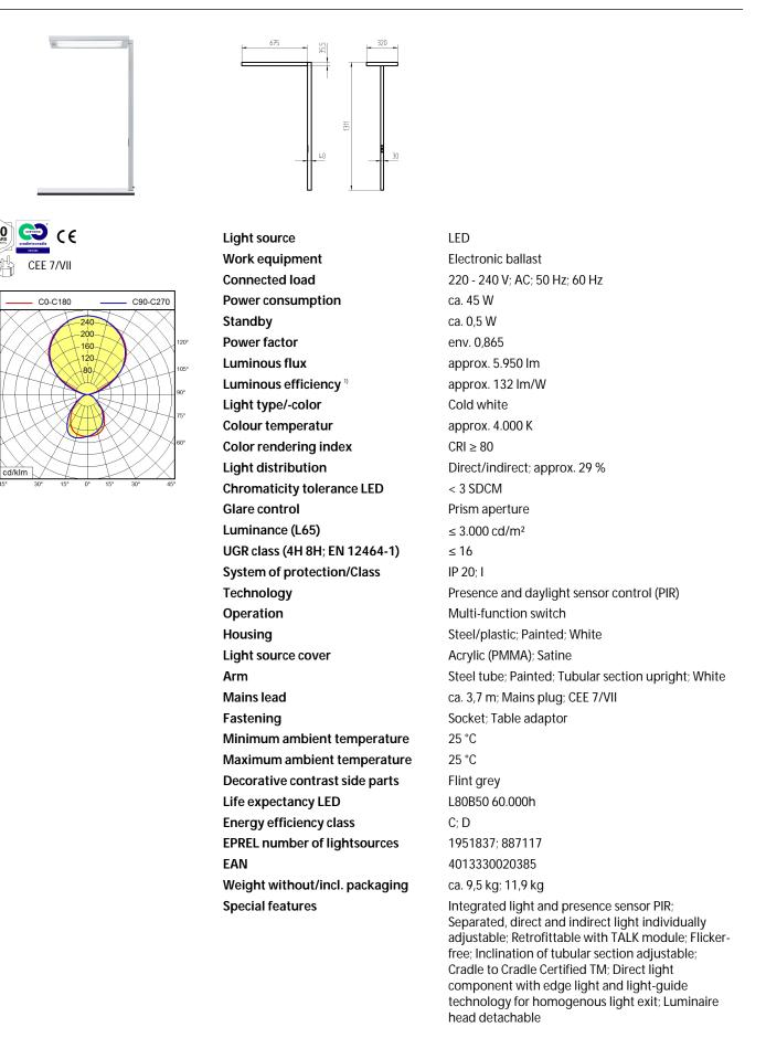
For luminaires with separate control gear, the luminous efficacy refers to the luminaire head without control g
