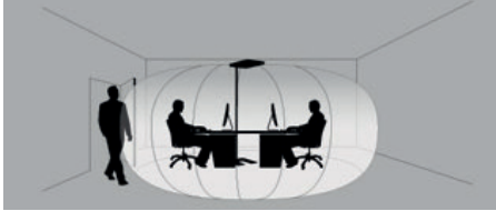
Fig. 18: Detection range of the HFMD.
