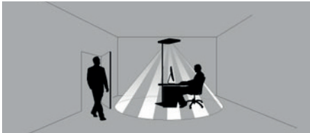
Fig. 19: Detection range of the PIR.
