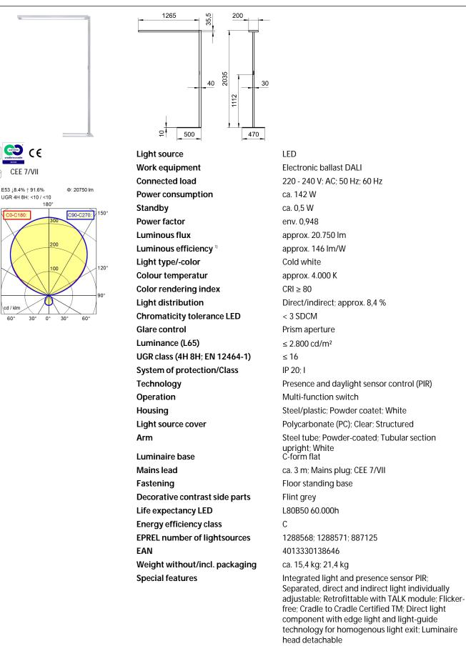
For luminaires with separate control gear, the luminous efficacy refers to the luminaire head without control g
