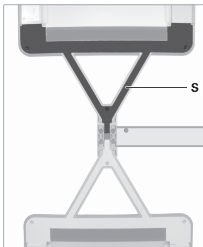
Fig. 24: Fitting the cover.
