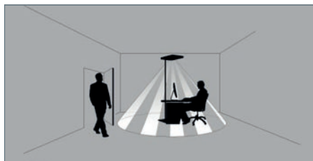
Fig. 31: Sensing range PIR sensor.
